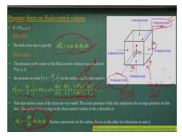
Now if I go for the next ones that how to get the pressure field when fluid is at the rest. That means I am just looking the what could be the functions of the P, P = P(x, y, z). If it that it is now again I am considering a very simple case, let us consider a control volume like this okay. This is what my control volume. As I said it when the fluid is at rest the shear stress become zero.
