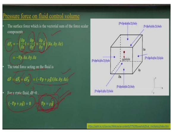
If I do that, that what as a vector form I can write it this way. This is the force component along the x directions. This is the force component along the y direction. This is a force component acting in the z direction. So this is a gradient vector. So I can have a gradient vector field of dF. As I said it earlier only two forces is there, one is a gravity force and another is force due to pressure distributions.
