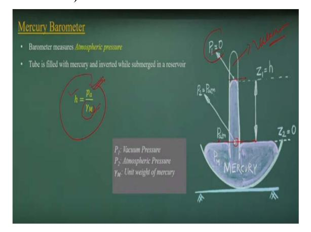
Now let me come it to the mercury barometer case with a very simplified same capability concept what we used to measure the atmospheric pressure. Here we use the mercury and just insert a tube such a way that the tubes would contain the vacuum. So we can have a system to remove the air and to have the vacuum and you just inserted in that tube on that one. Same concept again is coming it.
