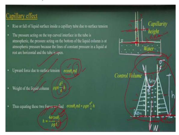
Now let me consider the capillary effect as you could have seen some of the books if any of the class 12th levels. What do we do it we just coming the two force components, the force due to the surface tensions and the gravity force of the capillary part. You know it what is the capillary. That means if use a small tube and insert it into a fluid, you can see there is a rise of water or the fall of mercury.
