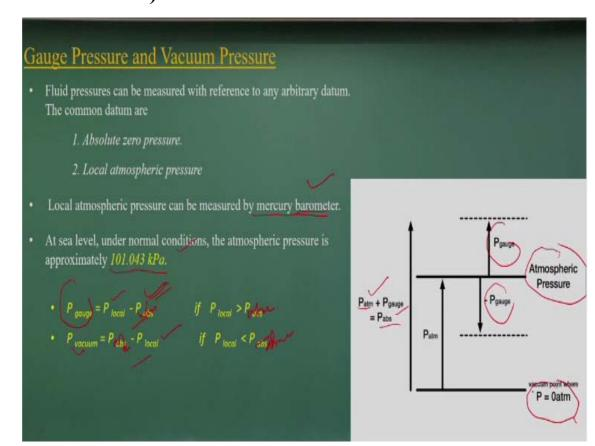
Now the point is what we are going to discuss is that gauge pressure and vacuum pressure. Components now is coming it what is your datum to measure the pressure. Whether you have to make a absolute zero pressure, that means you have a vacuum. From there you are measuring the pressure, or you consider as local atmosphere, to measure the pressure.
